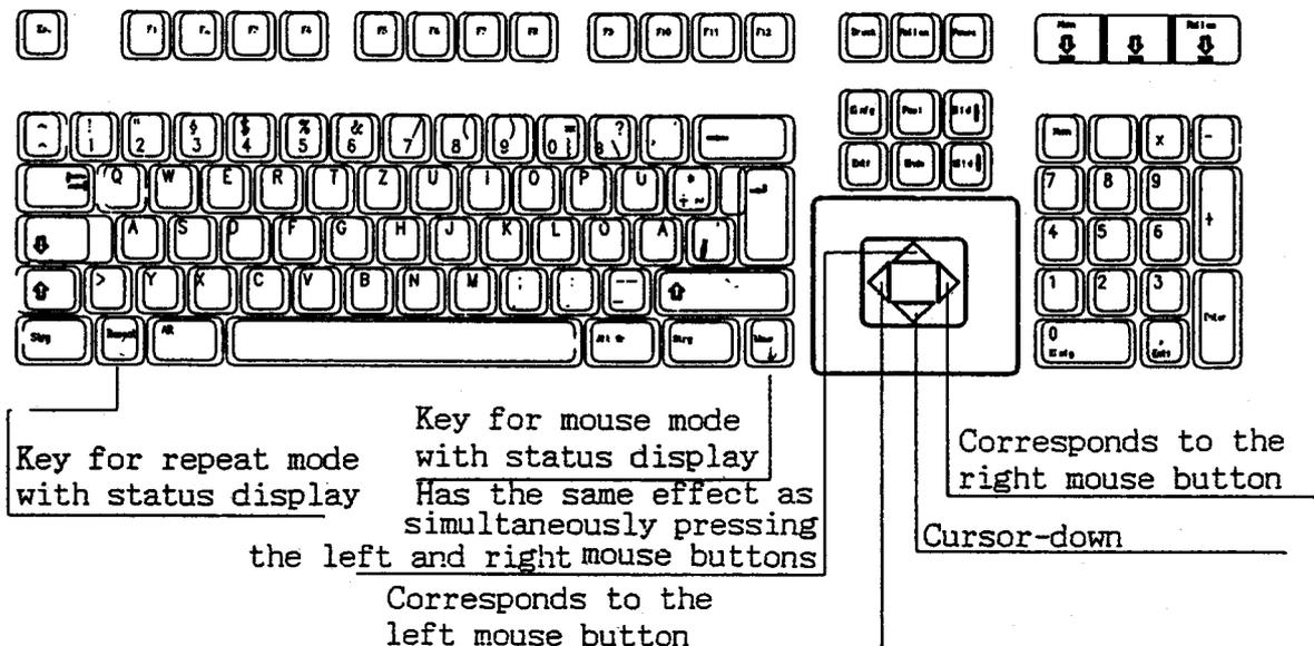
Text mode: In text mode, a further distinction is made between cursor and repeat mode. The four integrated buttons on the MouseBoard perform the same functions as the cursor keys in both cursor and repeat mode.
