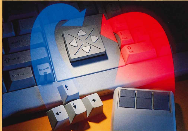
The integration of mouse and cursor functions into the Cherry MouseBoard eliminates separate mice and cursor keys.
