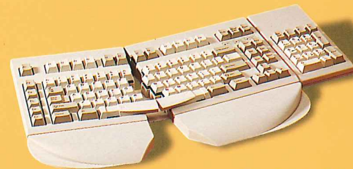
Frontal pitch of 12°; alphanumeric section horizontally adjustable between 0° and 30° in 5° steps.
