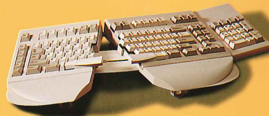
Raised to tent angle of 160°; alphanumeric section horizontally adjustable between 15° and 30° in 5° steps.
