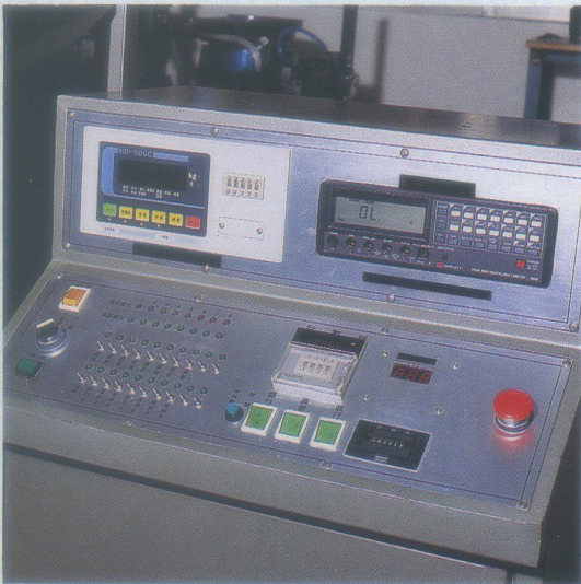
電腦自動化控制之鍵帽檢查裝置 Computerized inspection equipment of key-cap
